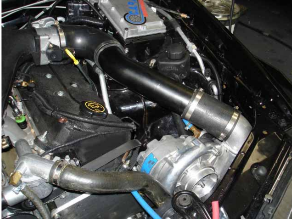
Photo 10: Discharge Pipe Fitment
