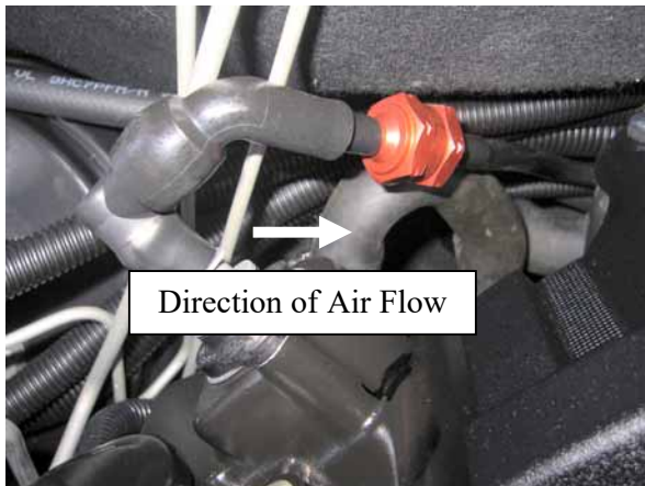
Photo 14: PCV Valve Mounting
