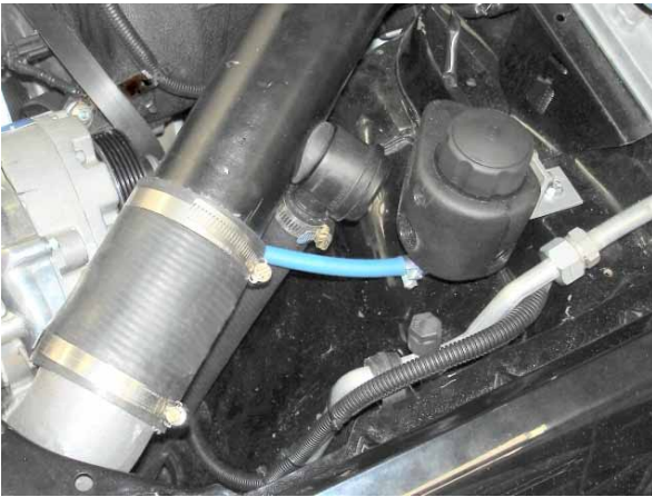
Photo 11: Blowoff Valve Fitment
