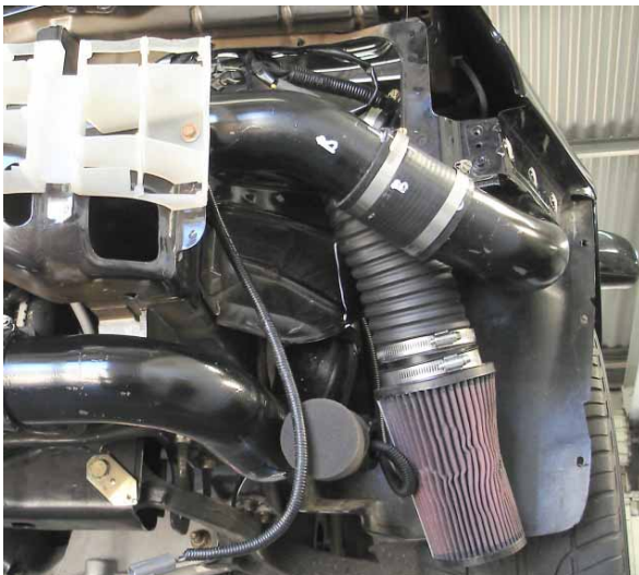
Photo 12: Intake Pipe Location
