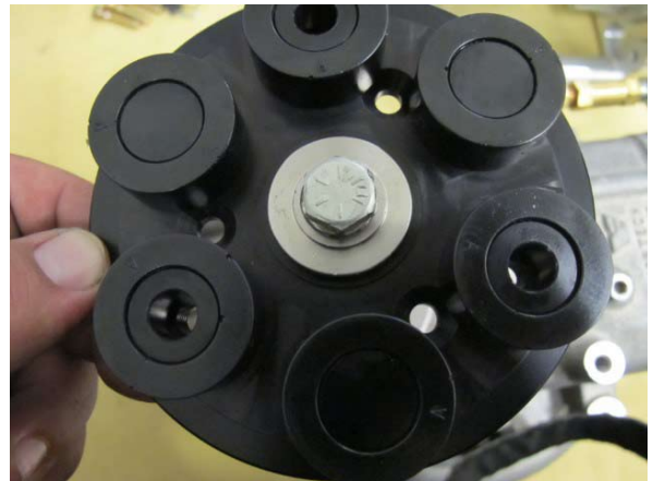
Fig. 7-b: Secure supercharger hub using provided screw and retainer
