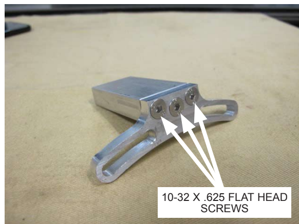
Fig. 4-a: Assemble crank trigger mount
