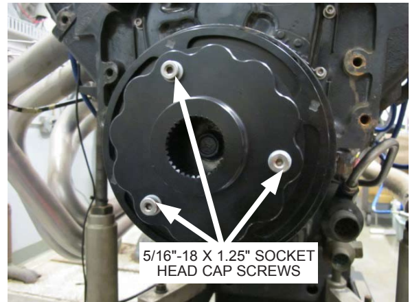
Fig. 3-d: Install crank hub cover
