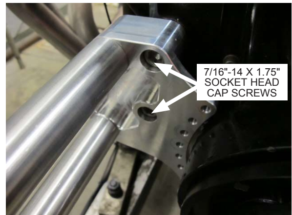
Fig. 5-b: Install both engine mount blocks
